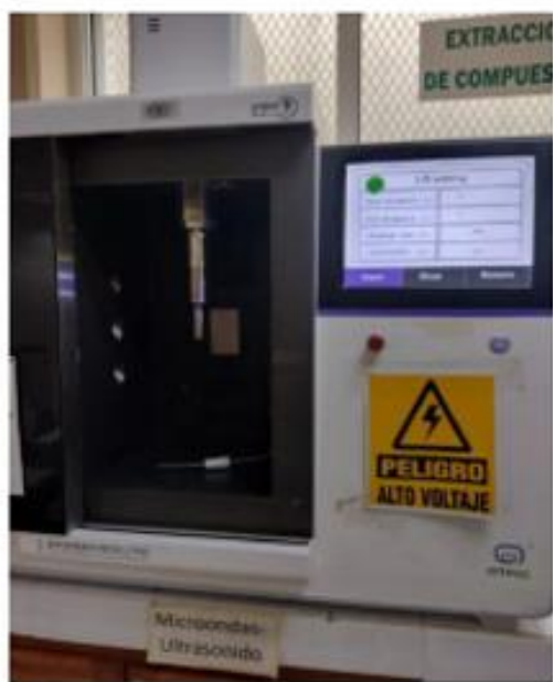
Figure 1. Microwave reactor (Ultrasonic Microwave Cooperative Workstation model XO-SM400).
